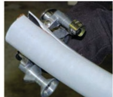
Teeth Gripping and Pulling Off Laminate Layer.
